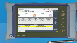
Modular Bi-directional Fiber Tester T-BERD 4000
